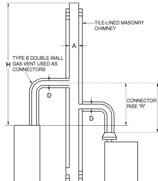
Table C504.3(3) is used when sizing Type B double-wall vent connectors attached to a tile-lined masonry chimney.
