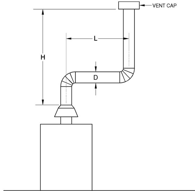
Asbestos cement Type B or single-wall metal vent serving a single draft-hood-equipped appliance [see Table C504.2(5)].
