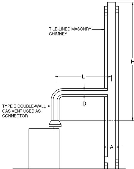
Table C504.2(3) is used when sizing a Type B double-wall gas vent connector attached to a tile-lined masonry chimney.
