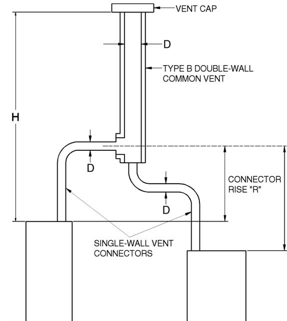
Table C504.3(2) is used when sizing single-wall vent connectors attached to a Type B double-wall common vent.
