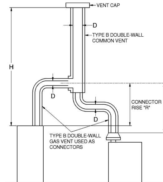
Table C504.3(1) is used when sizing Type B double-wall vent connectors attached to a Type B double-wall common vent.
