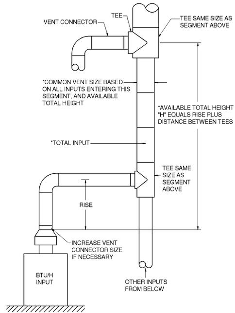
Vent connector size depends on: Common vent size depends on:
