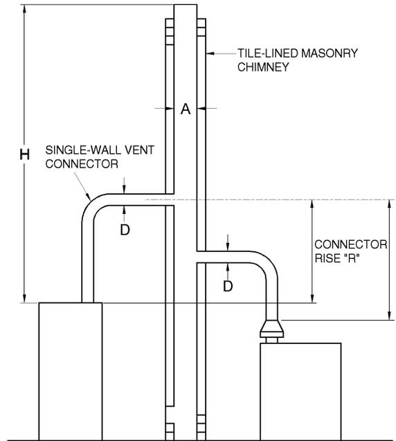
Table C504.3(4) is used when sizing single-wall metal vent connectors attached to a tile-lined masonry chimney.
