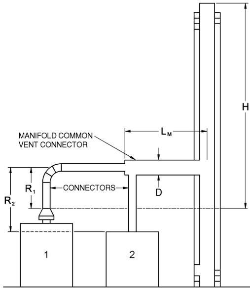
Example: Manifolded Common Vent Connector  $L_M$  shall be no greater than 18 times the common vent connector manifold inside diameter; i.e., a 4-inch (102 mm) inside diameter common vent connector manifold shall not exceed 72 inches (1829 mm) in length (see Section C504.3.4).
