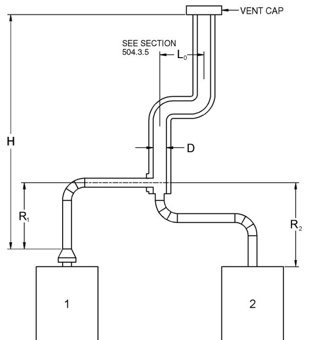
Asbestos cement Type B or single-wall metal pipe vent serving two or more draft-hood-equipped appliances [see Table C504.3(5)].
