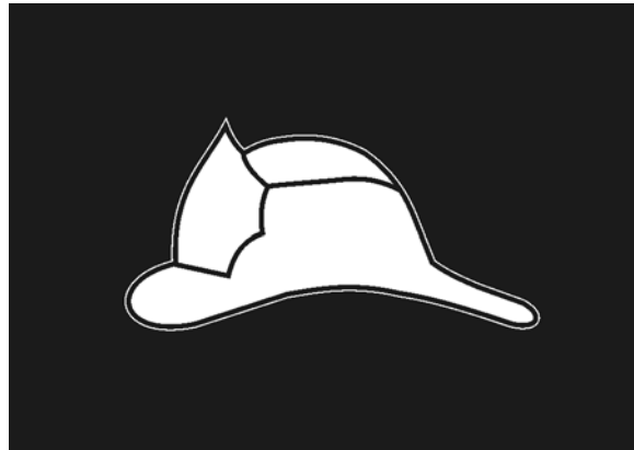
FIGURE 3007.7.5 FIRE SERVICE ACCESS ELEVATOR SYMBOL
