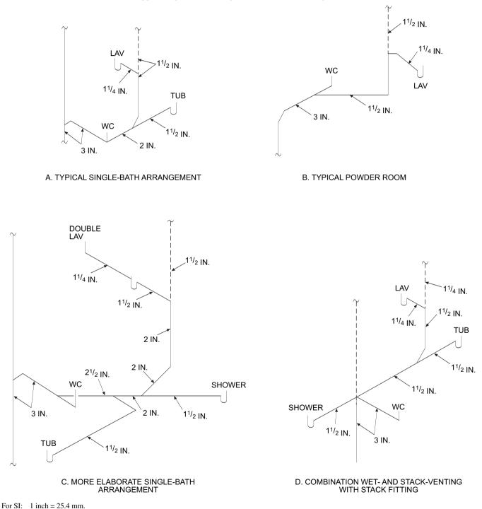
FIGURE N1 TYPICAL SINGLE-BATH WET-VENT ARRANGEMENTS
