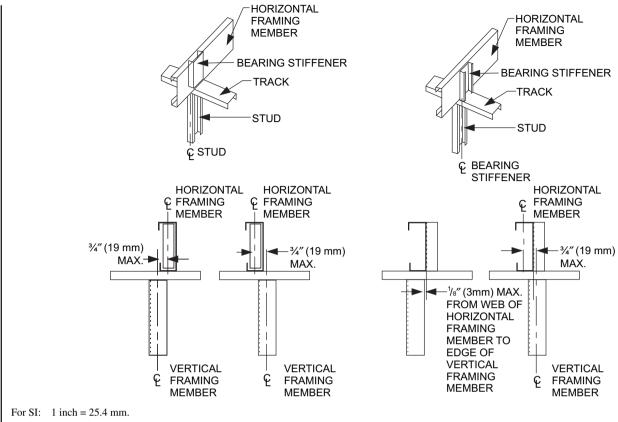
FIGURE R804.1.2 IN-LINE FRAMING
