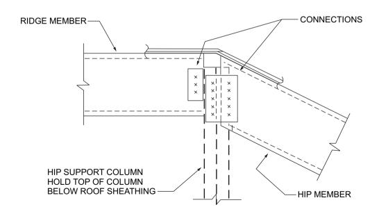
FIGURE R804.3.3.4(3) HIP CONNECTIONS AT RIDGE
